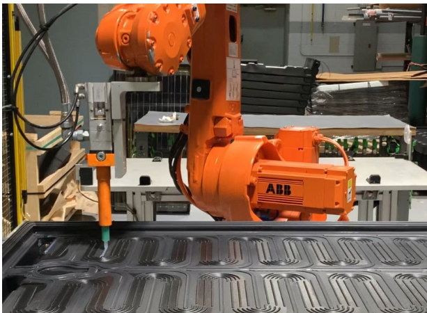
Robot applies adhesive in flat aluminized panel before solar cell placement
