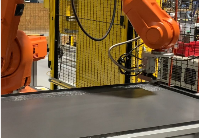
Robot applies adhesive in flat aluminized panel before solar cell placement
